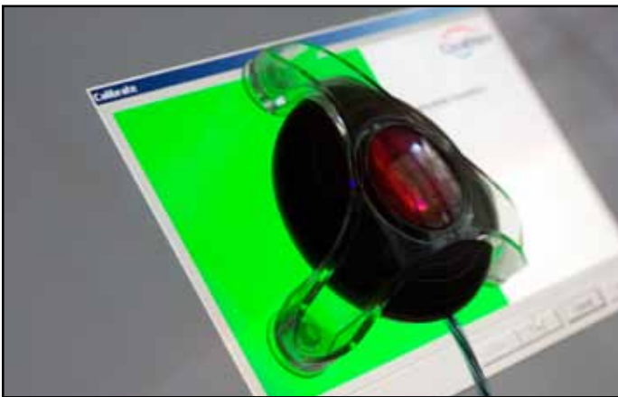
Colorvision (Pantone) "spyder" colorimeter attached to CRT monitor and sampling green light output. By measuring how the monitor displays colors it knows, the colorimeter software can calculate how far off your monitor is and make the necessary profile calibrations.
