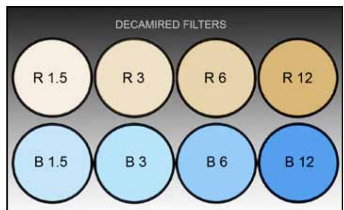
Decamired (MIREd) filters solve the problem of matching the light color to the film's requirements. Bluish tones correct light that is reddish and vice versa. European KR & KB filters are based on MIREd values.
