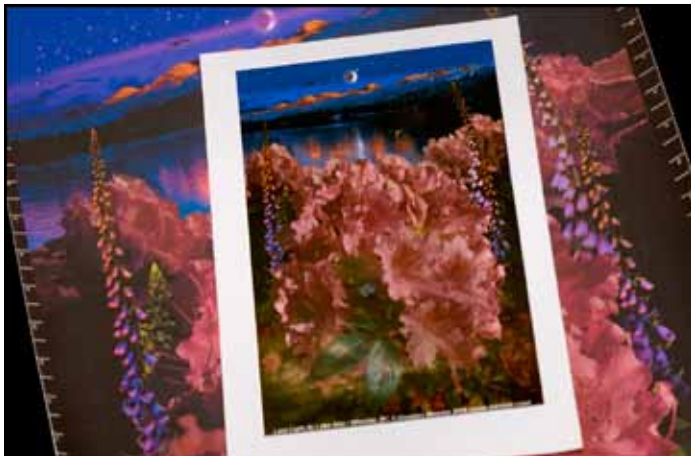
The wider tone range revealed by gloss finishes can be clearly seen in this comparison of Epson Glossy Paper and Matte Canvas. Matte finishes make "scatter light" which lightens dark tones, killing contrast.
